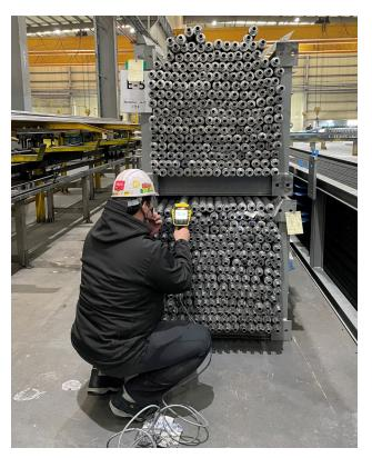
Therefore, it was decided to proceed with the visual test using the bore-scope, but it took too much time and the production schedule was disrupted afterwards, so a quick and accurate inspection method was found.
