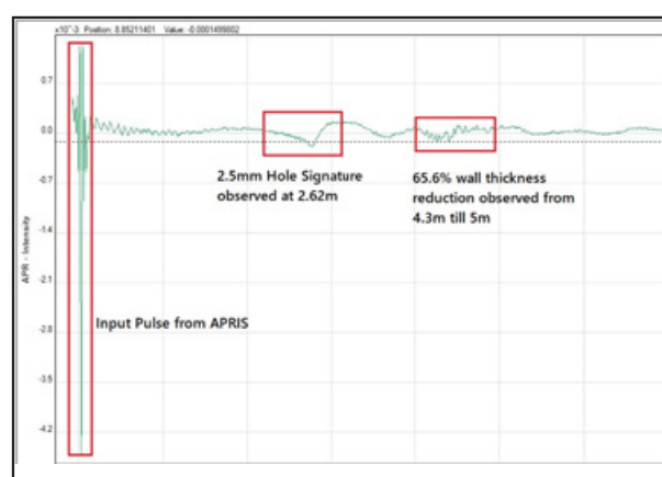
Figure 5: Graphical representation of defects detected.
