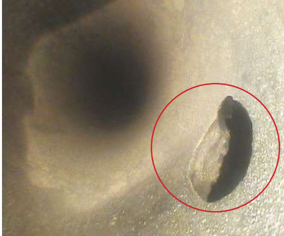
Figure 3: APR Tube #1, 3.3mm hole at 9.66m
